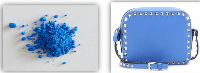
Sl.26. Kobaltov(II) aluminat, \text{CoAl}_2\text{O}_4 , kao plavi kobaltov pigment [41,42]
