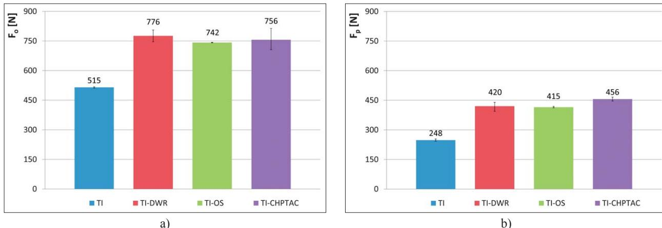
Fig.4 Breaking force of printed waste cotton fabric before and after cationization: a) warp direction ( $F_o$ ) and b) weft direction ( $F_p$ )
