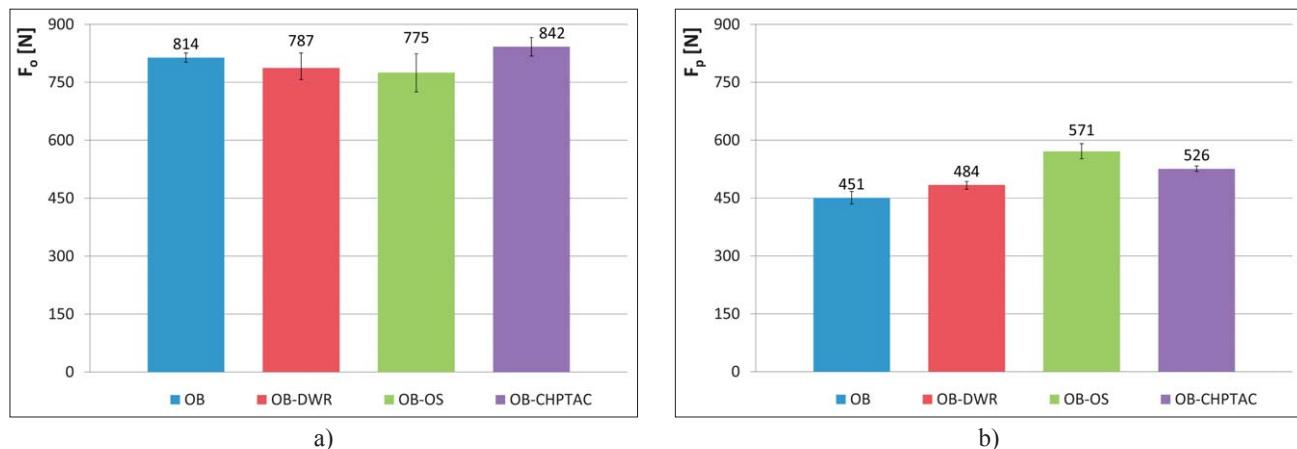
Fig.2 Breaking force of optical brightened waste cotton fabric before and after cationization: a) warp direction ( $F_o$ ),
