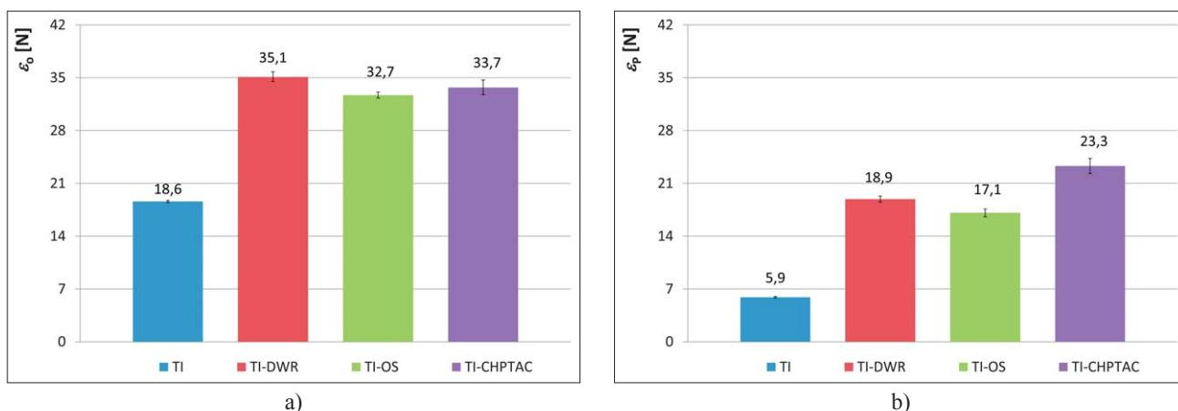
Fig.5 Breaking elongation of printed waste cotton fabric before and after cationization: a) warp direction ( $\varepsilon_o$ ) and b) weft direction ( $\varepsilon_p$ )
