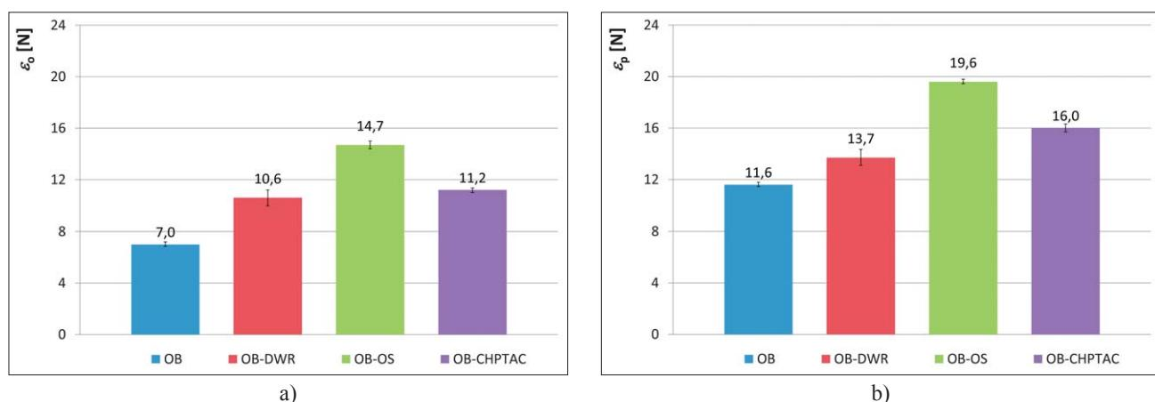
Fig.3 Breaking elongation of optical brightened waste cotton fabric before and after cationization: a) warp direction ( $\varepsilon_o$ ),
