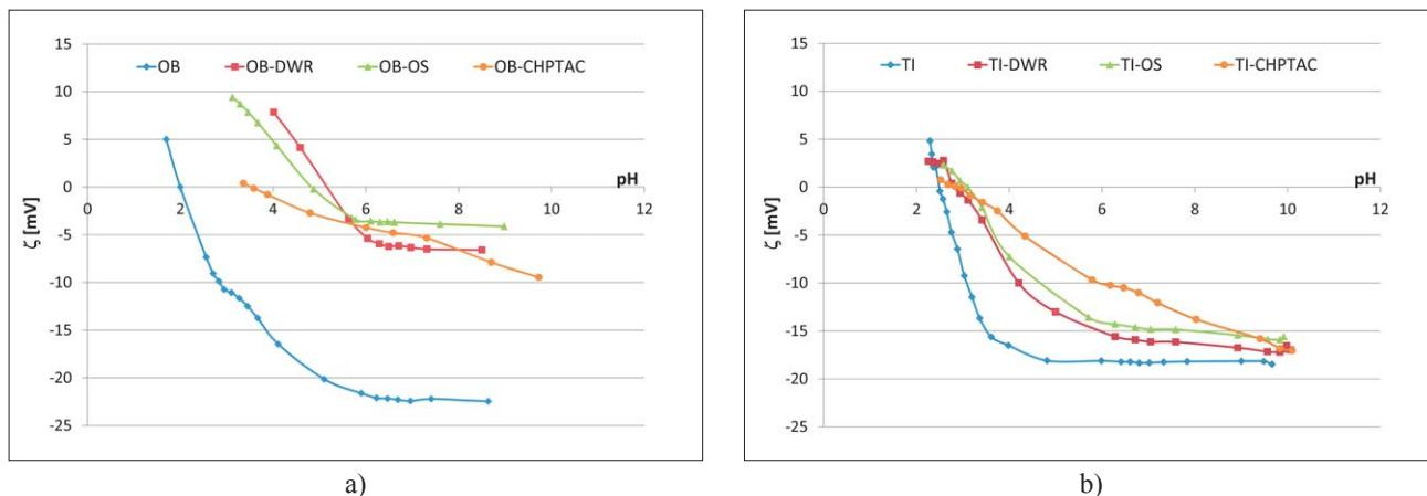
Fig.1 Zeta potential ( $\zeta$ ) of waste cotton fabric before and after cationization in dependence of pH of electrolyte 0.001 M KCl:
