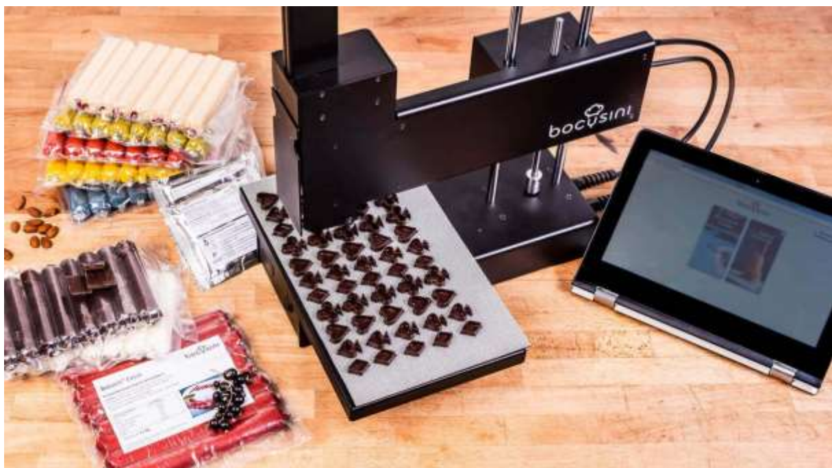
Sl. 5. The Bocusini 3D printer hrane [11]
