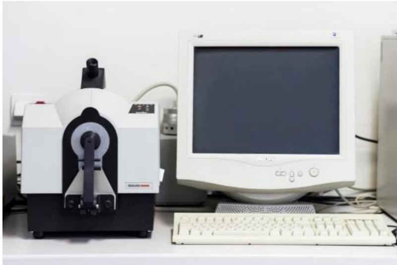
Sl. 44. Spektrofotometar DataColor Spectra Flash 600 PLUS-CT [14]
