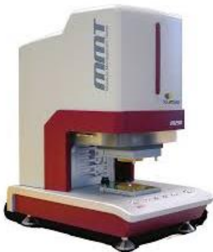
Slika 29. Moisture Management Tester M290, SDL [68]
