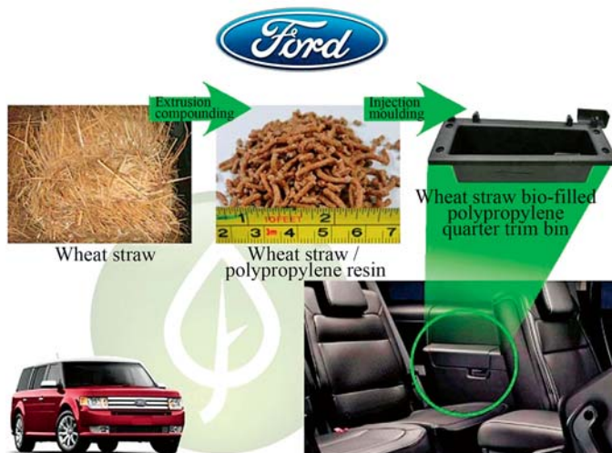
FIGURE 15 – Bioplastics made from wheat straw and polypropylene 51
