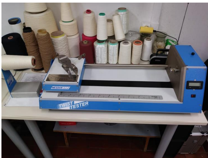
Sl. 20. Torziometar, Twist –T, Mesdan Lab
