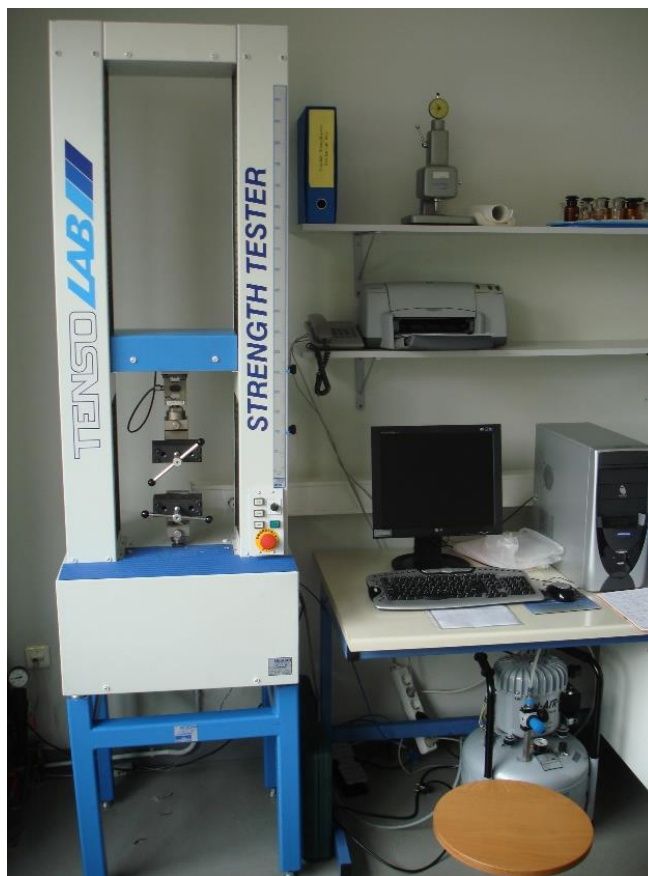
Sl. 18. Dinamometar Tensolab 1000/3000 - Mesdan Lab
