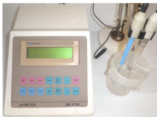
Slika 25: pH metar, Metrel
