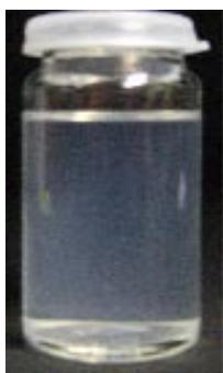
**Figure 1.** Image of a ZnO-sol taken 10 weeks after synthesis. The absence of any precipitation proves the excellent stability of the colloidal solution.
