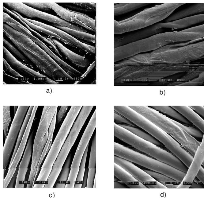
**Figure 5.** SEM micrographs of: (a) blank cotton fabric, (b) cotton fabric treated with 20% nano-ZnO, (c) blank cotton/polyester fabric and (d) cotton/polyester fabric treated with 20% nano-ZnO.
