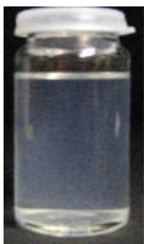
Figure 1. Image of a ZnO-sol taken 10 weeks after synthesis. The absence of any precipitation proves the excellent stability of the colloidal solution.
