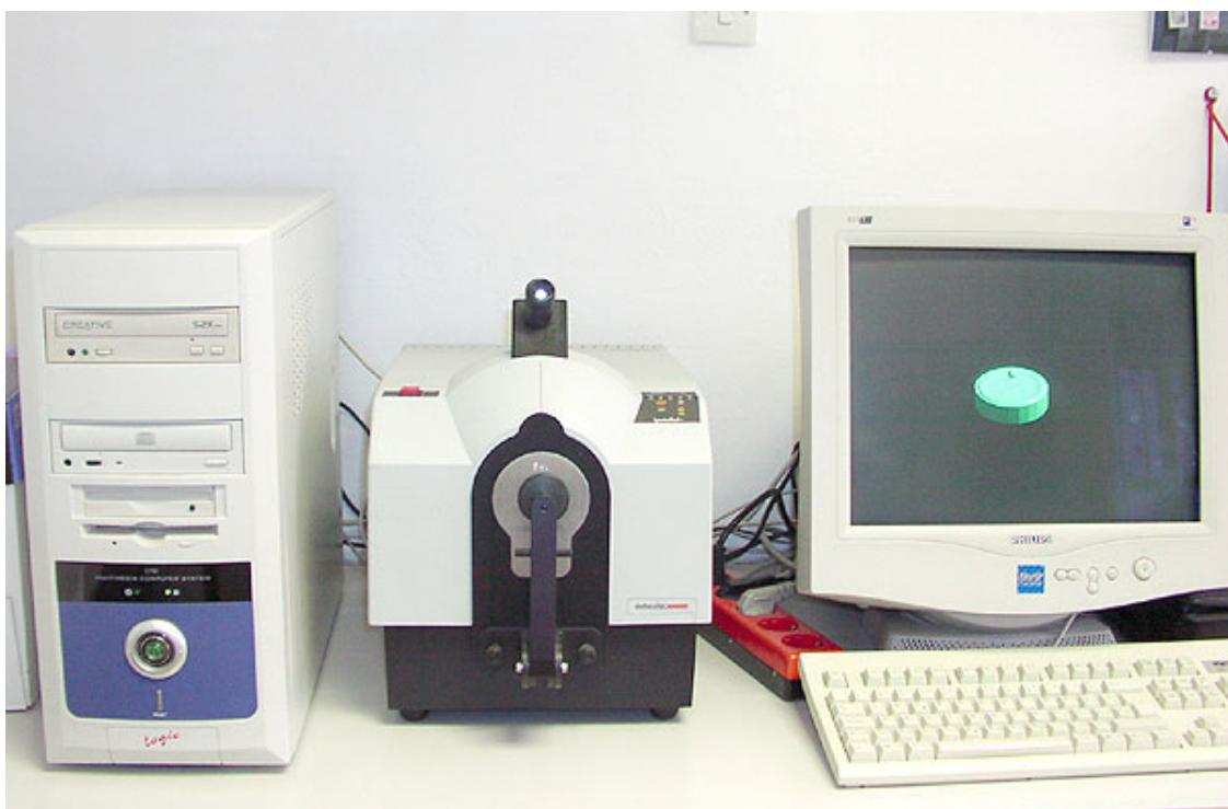
**Slika 18.** Datacolor remission spectrophotometer Spectraflash SF 600 PLUS CT
