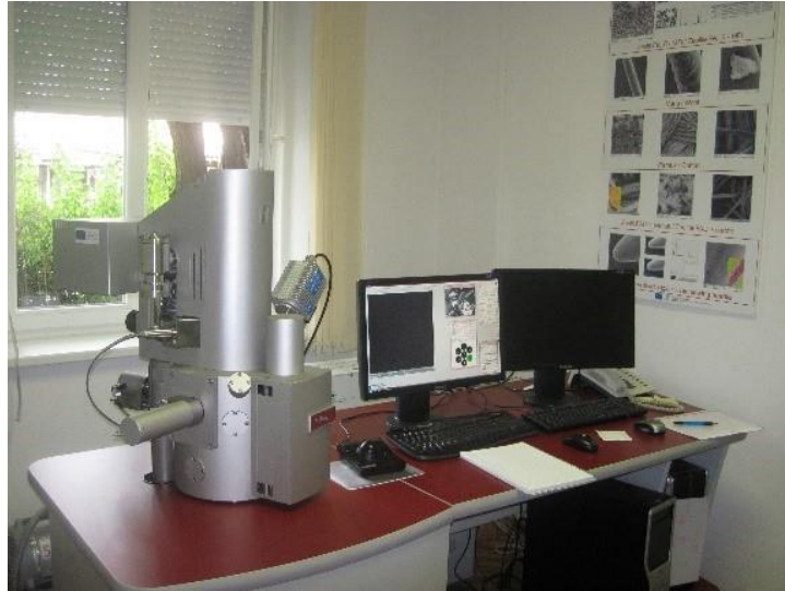
Figure 19: SEM-EDS, Tescan – Oxford Instruments
