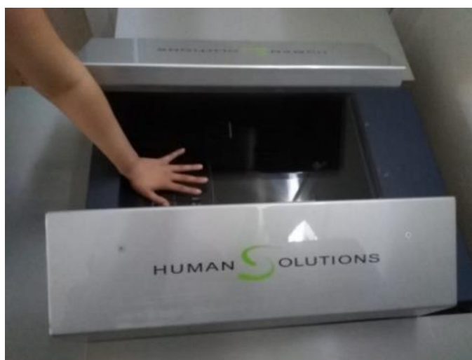
Slika 13. 3D skener tt. Human Solutions [6]
