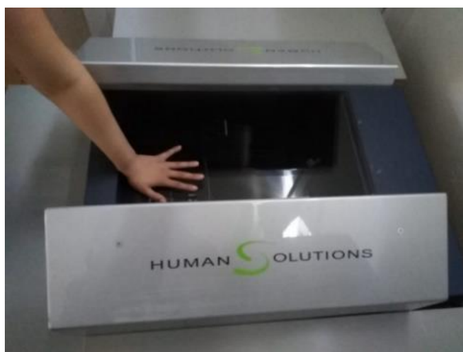
Slika 13. 3D skener tt. Human Solutions [6]
