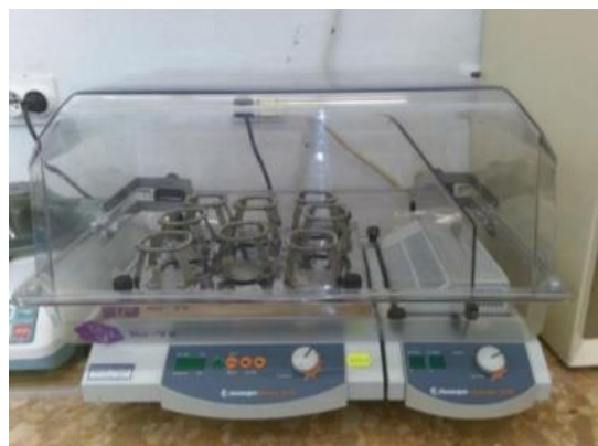
Sl. 12 Mućkalica Heidolph Unimax 1010 i Heidolph Inkubator 1000
