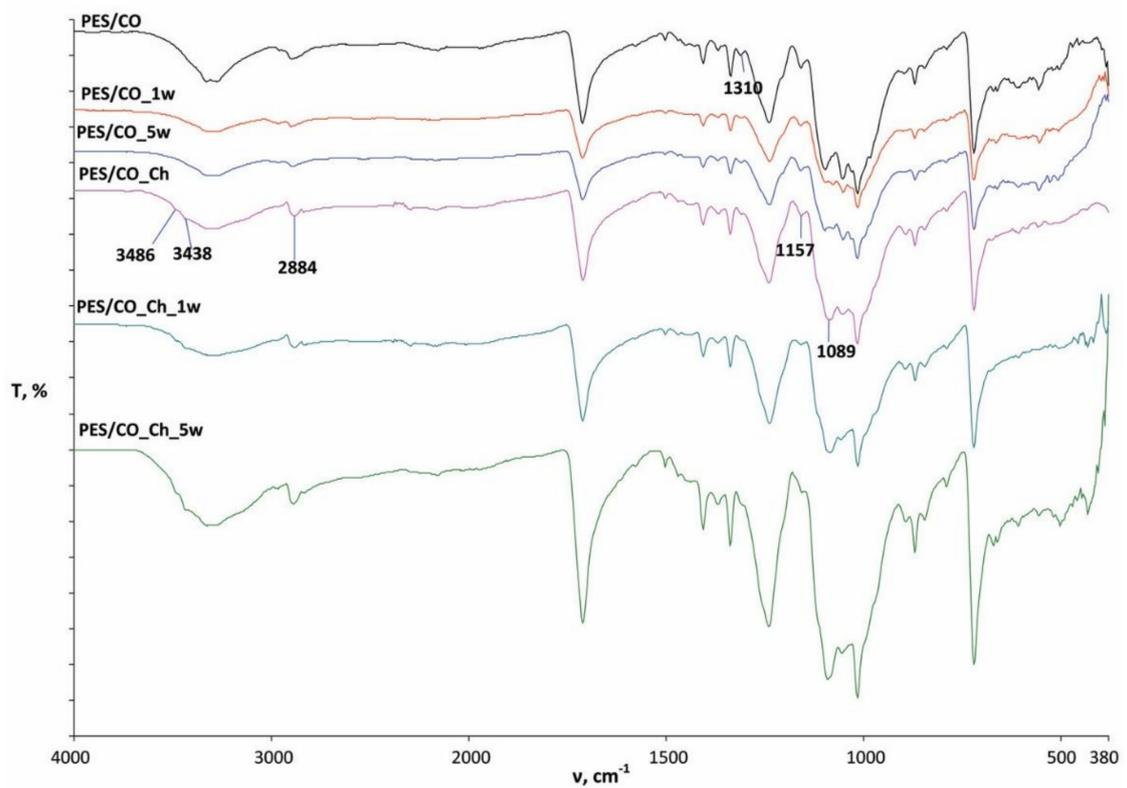
**Figure 7.** Polyester/cotton (PES/CO) blend fabric and the spectral bands of the treated samples (PES/CO\_Ch) and after first (PES/CO\_1w, PES/CO\_Ch\_1w) and fifth washing cycle (PES/C\_5w, PES/CO\_Ch\_5w).
