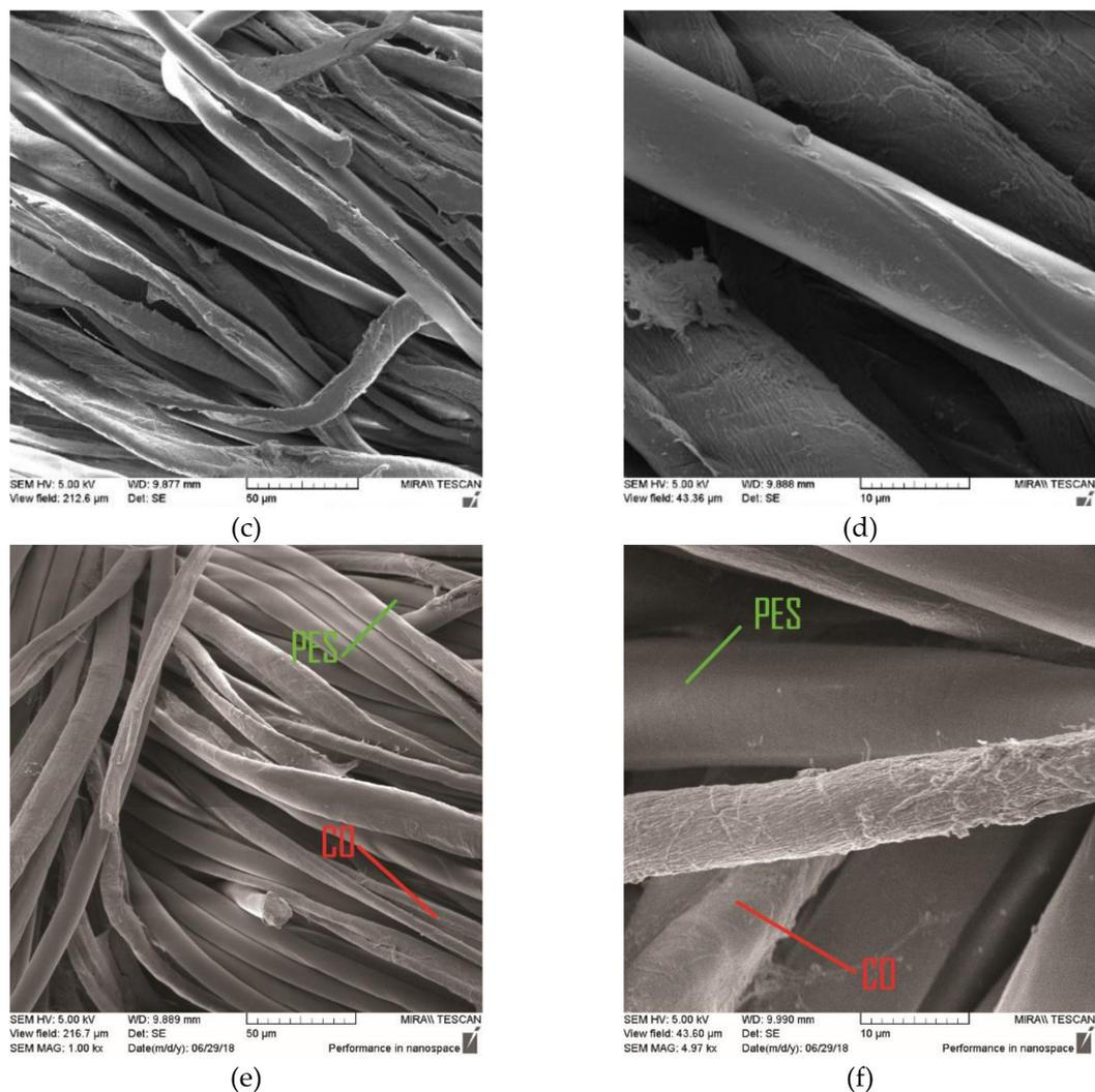
**Figure 4.** The SEM images of polyester/cotton fabric (PES/CO) with implemented chitosan: (a, b) before (PES/CO\_Ch); (c, d) after one washing cycle (PES/CO\_Ch\_1w) and (e, f) after five washing cycles in magnifications of (a, c, e) 1000 $\times$ , and (b, d, f) 5000 $\times$ .
