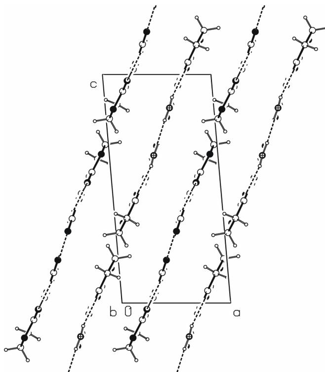
The crystal packing diagram along *b* axis (Figure 4) reveals that the hydrogen-bonded chains are parallel to the  $(\bar{2}, 0, 1)$ . The distance between the planes passing through the center of the hydrogen-bonded molecules is approximately 3.05 Å. Very similar one-dimensional hydrogen-bonded chains generate N–H···O hydrogen bonds in 1-carbamyliminomethylenetetrahydropyrrol-2-one [19].
