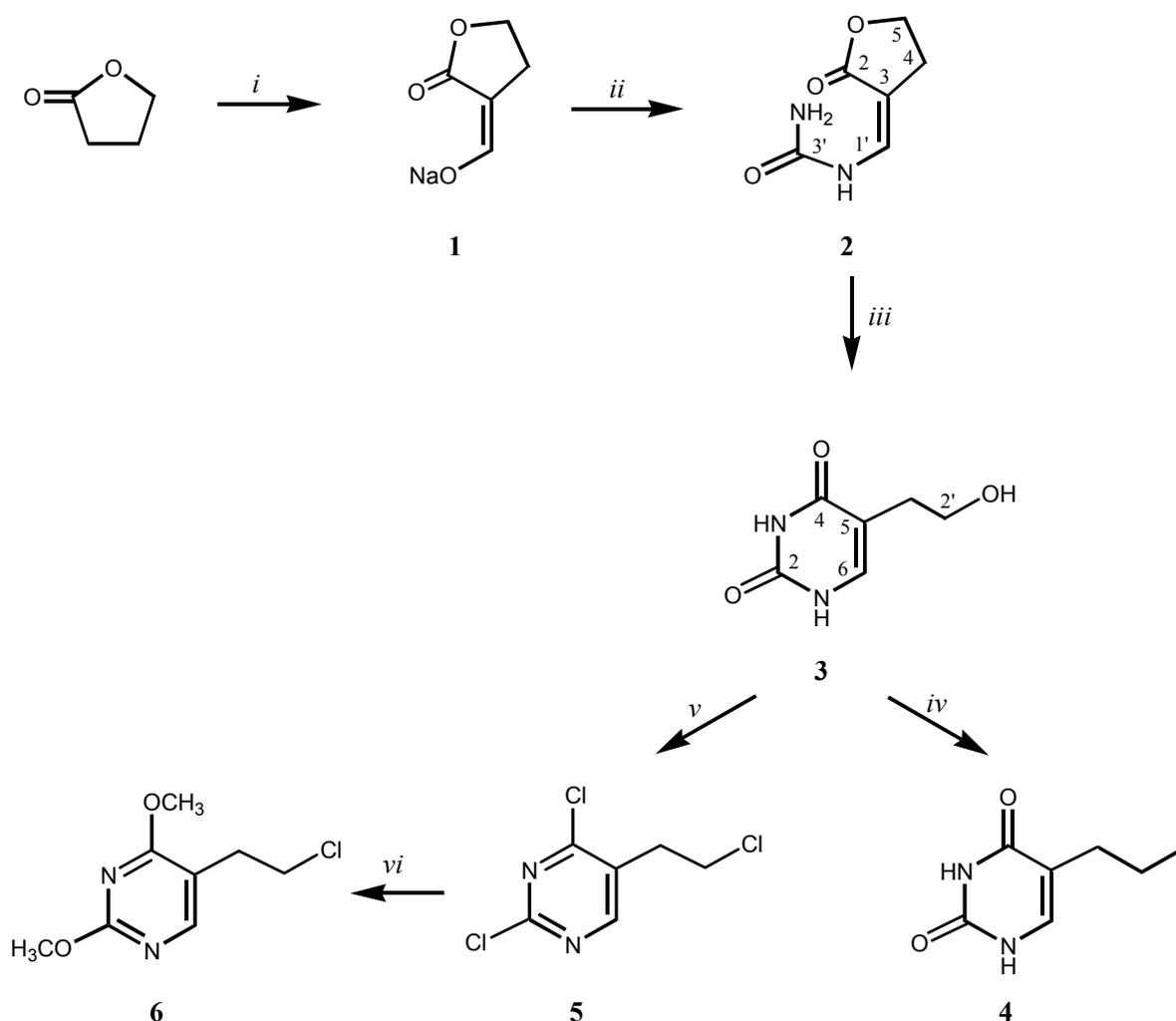
*Reagents and conditions:* (i) NaOMe, ether, HCOOCH<sub>3</sub>, 24 h; (ii) urea, 3M HCl, 4 °C, 24 h; (iii) NaOEt, ethanol, reflux, 6 h; (iv) HI, -5 °C, 90 min; (v) POCl<sub>3</sub>, reflux, 1h; (vi) NaOMe, reflux, 6 h.
