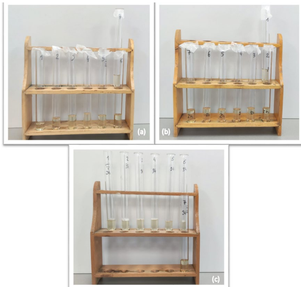
Slika 23. Alikvoti otopina vlakana obrađeni proteazom – (1) m.o., (2) 1%, (3) 0.5%, (4) 0.2%, (5) 0.1, (6) 0.05%, (7) 0.01%; nakon (a) 1h, (b) 2h i (c) 3h
