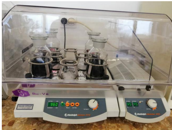
Sl. 14. Mućkalica Heidolph Unimax 1010 i Heidolph inkubator 1000
