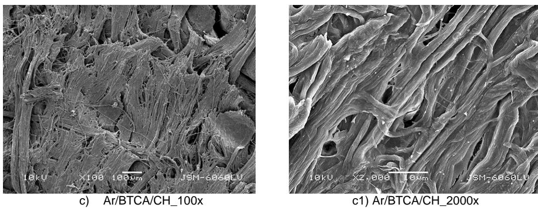
**Slika 51.** SEM snimke cjepanika (Cr štava) uz povećanja 100x i 2000x: a) i a1) argonova plazma; b) i b1) obrada Ar/CH; c) i c1) obrada Ar/BTCA/CH
