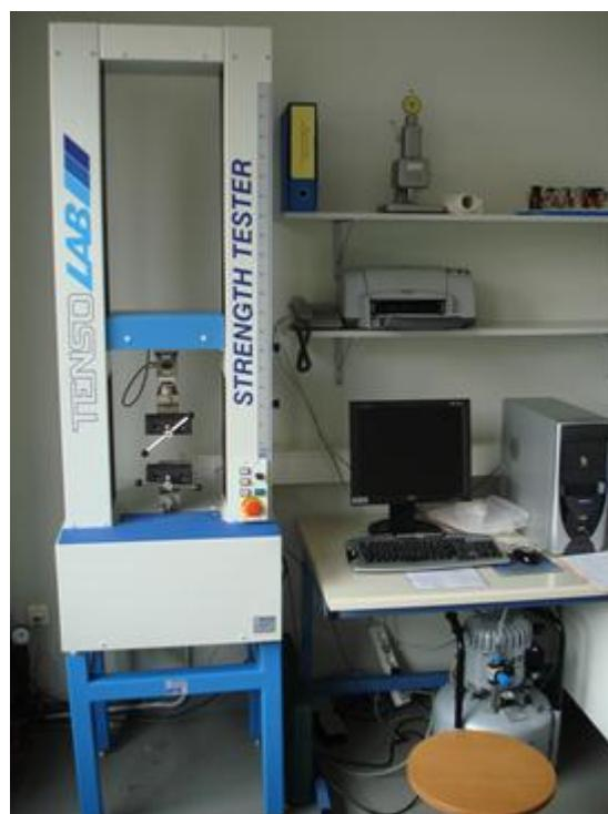
Slika 3. Dinamometar Tensolab 1000/3000 – Mesdan Lab
