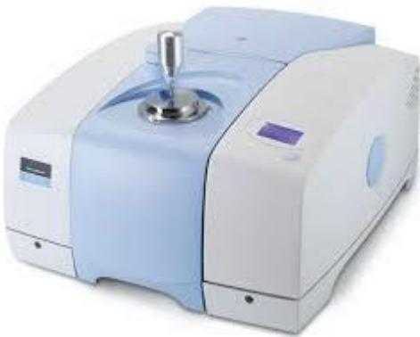
Slika 13: Perkin Elmer Spectrum 100 FTIR-ATR [27]
