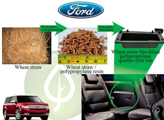
FIGURE 15 – Bioplastics made from wheat straw and polypropylene 51
