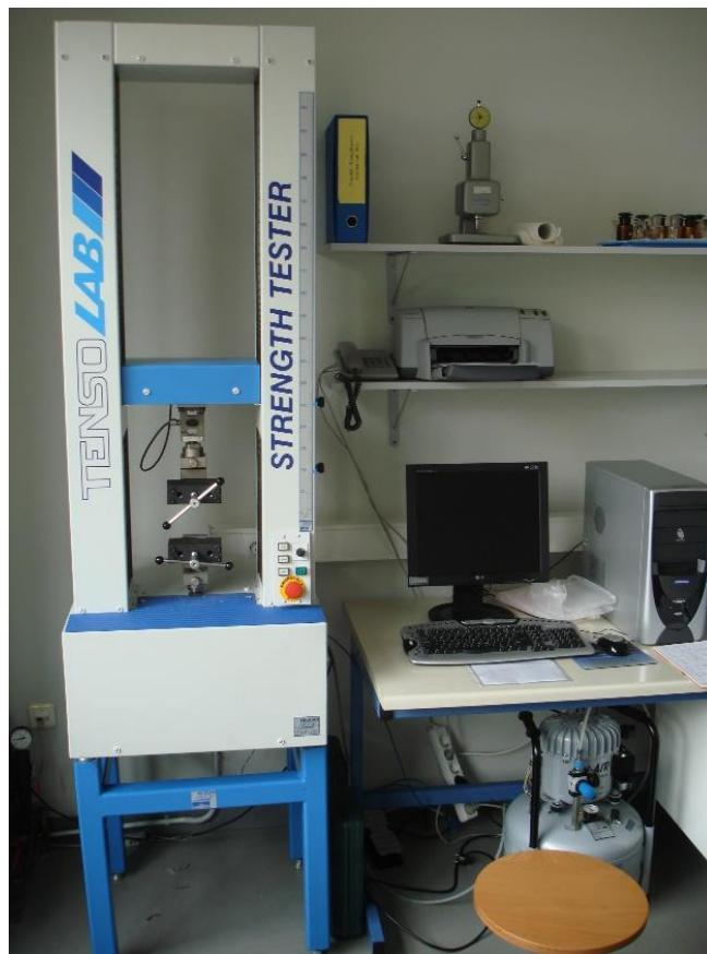
Sl. 18. Dinamometar Tensolab 1000/3000 - Mesdan Lab
