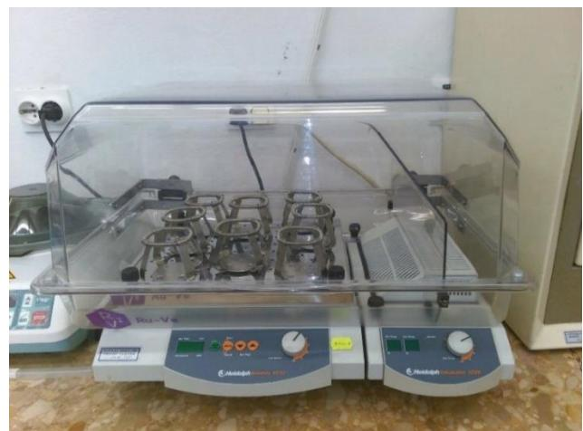
Sl. 14 Mućkalica Heidolph Unimax 1010 i Heidolph Inkubator 1000
