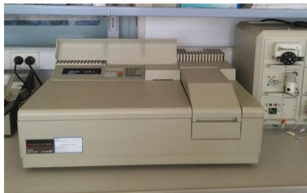
Sl. 11 Spektrofotometar Lambda 20, Perkin Elmer
