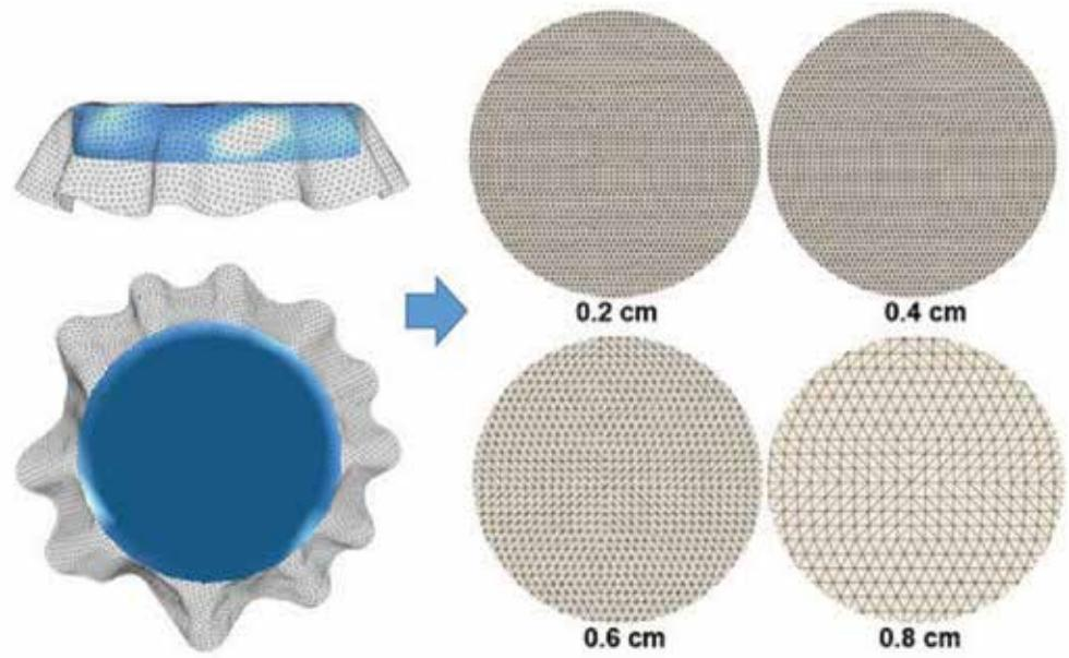
Computer circular fabric samples with different polygonal mesh densities,
