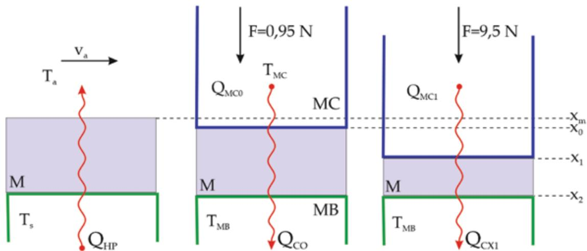
Measurement of characteristic parameters on hot plate and
