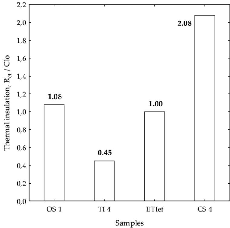
Presentation of the thermal insulation efficiency parameter (ETIef) calculated from the value of the thermal insulations of the clothing system (CS) and the outer shell (OS)
