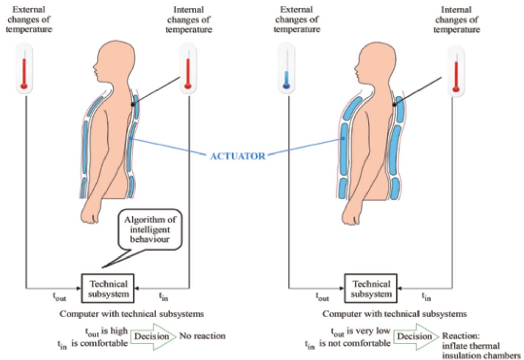
**Working (action) of the adaptive thermal insulation chambers as an actuator in intelligent clothing when external or internal temperatures changes**
