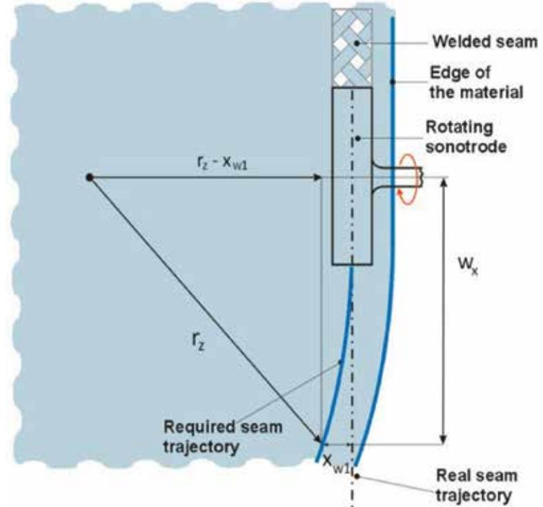
Layout of welding two layers of polymer materials with rotary ultrasonic sonotrode together with the specified technological welding parameters
