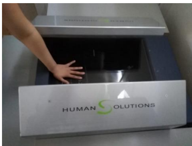
Slika 13. 3D skener tt. Human Solutions [6]
